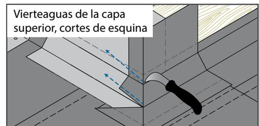
Base Flashing on Parapet Wall, Outside Corner
